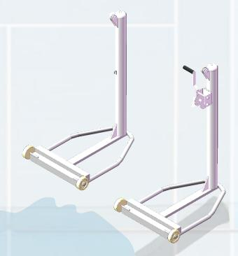
The base where the posts are welded is compound of a tubular profile joined to the back where the counterweights are welded ensuring the fixation of the posts. Moreover, these counterweights have wheels to facilitate their transport.
