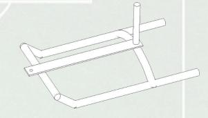
bracket and enough dimensions to place weight discs with different sizes, and with a fastening point to place the drag strip that will be attached to the waist.
