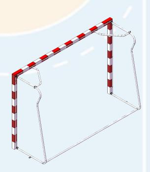
The stabilizer system is composed on the one hand of lateral supports (arches) attached to the frame at the top and bottom with a novel system formed by a metal die with screw that allows regulation to ensure the perpendicularity of the frame and fold the structure so that it occupies a minimum space in transport and packaging, and on the other hand, to ensure rigidity and stability, upper and lower stiffeners are placed between the arches.
